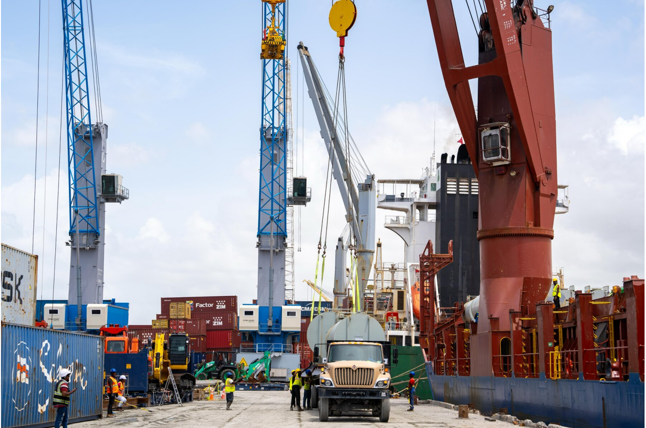
Shore cranes and ship gear working in tandem to discharge transformer cargo at the port of Georgetown.
