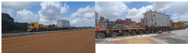
The 18-axle Goldhofer trailer en route along the access road, and staged at the port yard ahead of onward transport.
