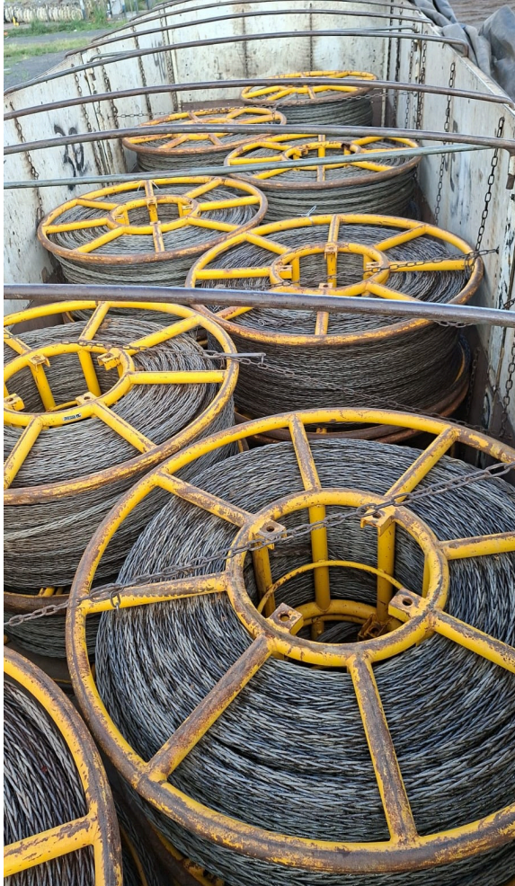
Steel wire-rope reels grouped and secured for inland transport.
