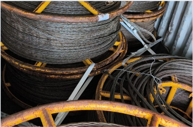
Wire-rope reels restrained inside an enclosed container.
